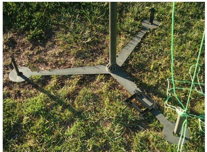
Base of the military surplus fiberglass mast holding up the G5RV Jr.
