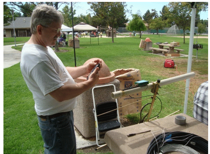
Gary WB6YRU gets ready to run a transmitter hunt. Here he puts a paperclip into the antenna port of a handheld to attenuate the signal (since the transmitter is so close). Note the handheld beam leaning up against the table.
